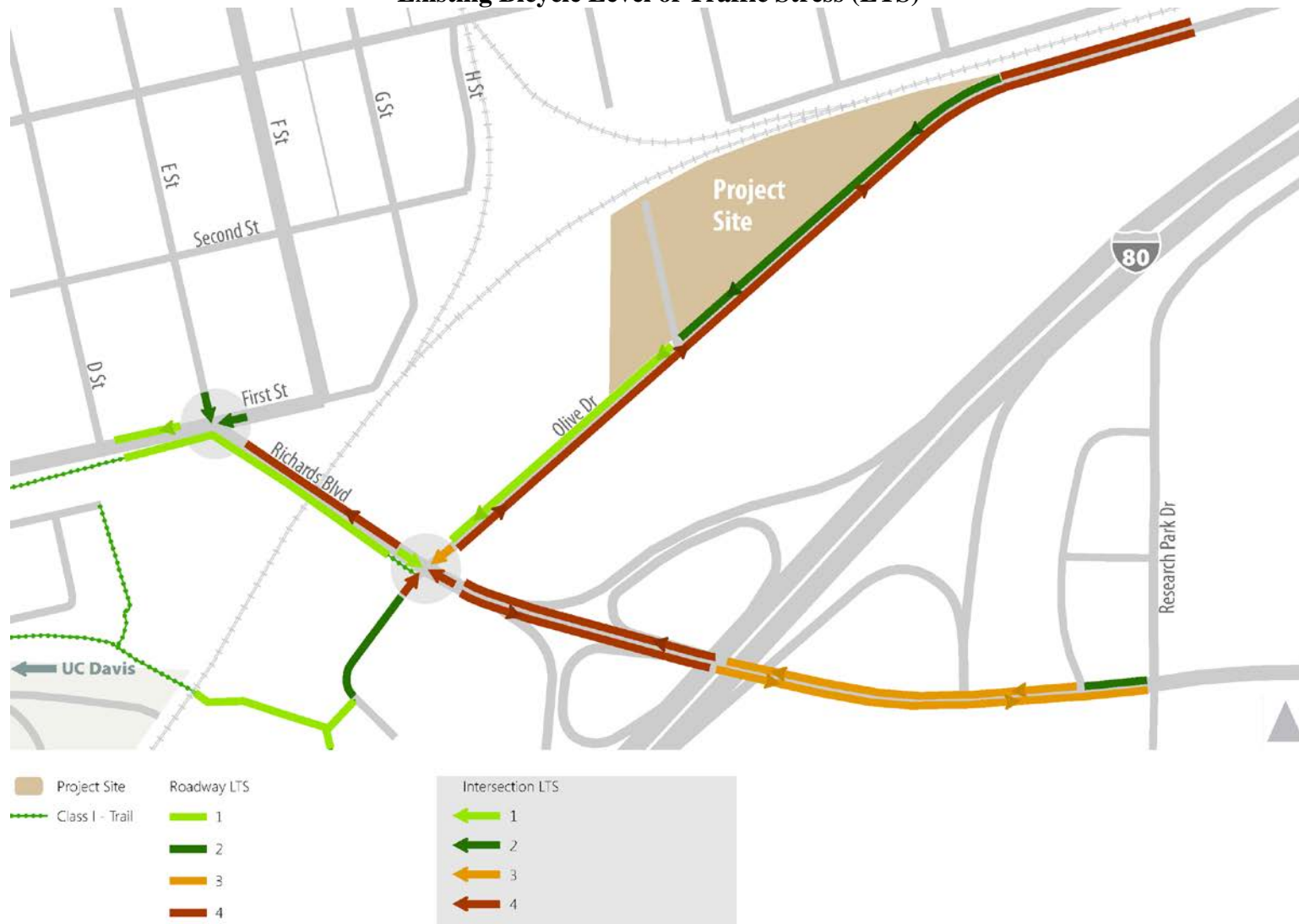
Figure 4.11-5 Existing Bicycle Level of Traffic Stress (LTS)
